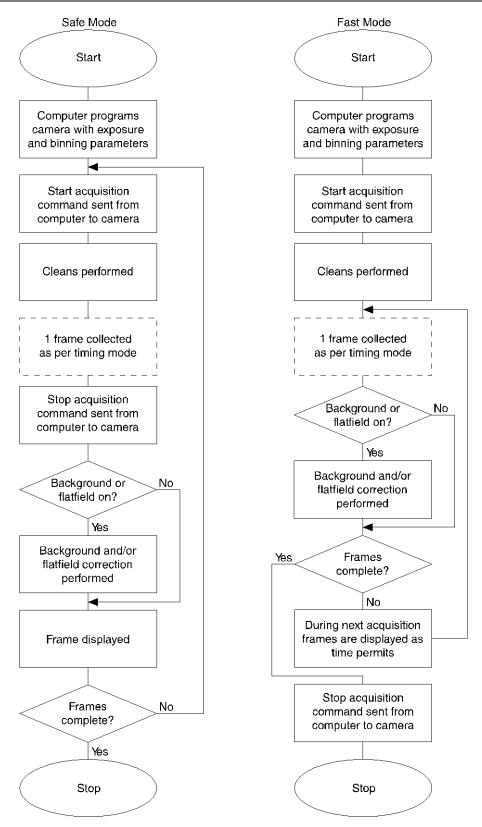
Figure 21. Chart of Safe Mode and Fast Mode Operation
